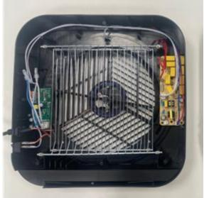
Carefully replace the rear cover ensuring it is flat, square and correctly aligned.
