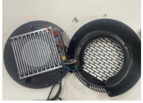
Remove the rear cover. There is sufficient cable length to place the rear cover next to the top cover without disconnecting the terminals.
