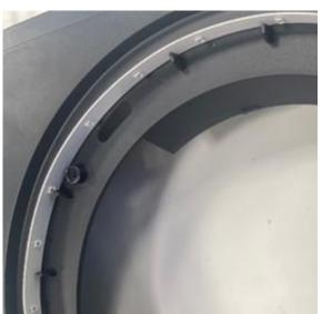
Install the replacement LED strip. Ensure that the strip sits behind the upstands and seated correctly. Connect the LED strip light connector to the wire. Carefully refit the diffuser assembly, ensure it is aligned correctly and flat to the body.
